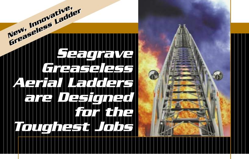
Seagrave aerial ladders are made for flawless performance — even in the most challenging conditions. And now our ladders feature new Polygon greaseless bushings with over twice the compressive strength of bronze — providing superior durability during the toughest calls and rescues.
